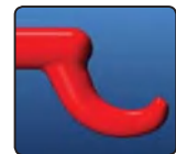
Optimum gate geometry, with edges rounded
