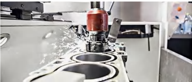
Die & Mould Components Production Facility - Precise Honing Machines with Pneumatic Measurement Systems
