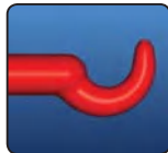
Optimum gate geometry, with edges rounded
