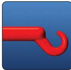
Optimum gate geometry, with edges rounded
